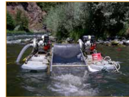
Suction dredgers (above) use a gas-powered engine to suck the river bottom up, sift it for gold, and spew sediment into the water column (above top). Photos by Scott Harding and Mid Klamath Watershed Council.
