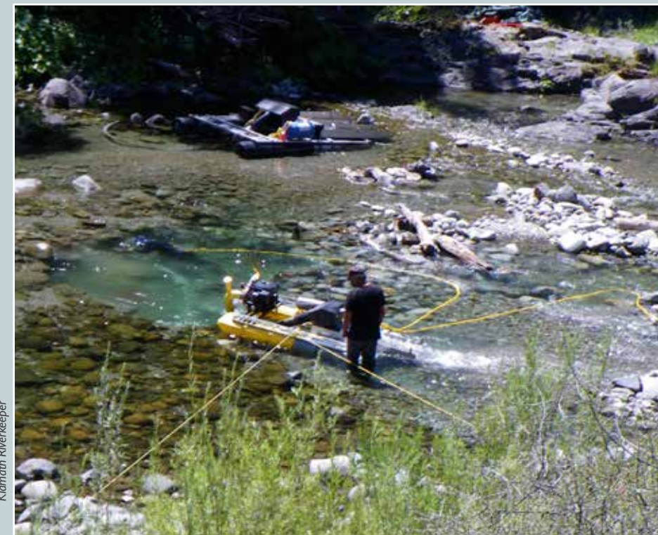
A small illegal suction dredge mining operation on the Scott River in the Klamath watershed in 2009. The suction intake can be seen sucking up gravels beneath the water to the left of the dredger. Dredgers can run twice this size powered by two gas motors.
