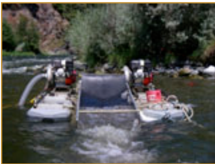
Suction dredgers (above) use a gas-powered engine to suck the river bottom up, sift it for gold, and spew sediment into the water column (above top). Photos by Scott Harding and Mid Klamath Watershed Council.
